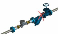
2. It is recommended that at least one side of meter will be connected to a PVC (or plastic) pipe.
