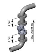
2 pipe diameters before and after elbows (90°) in vertical installations
