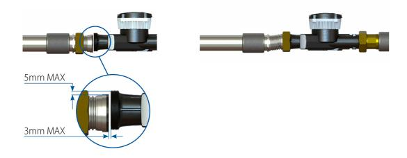
6. Please start to tighten the end connections by hand. Final tightening will be with no more than 100Nm torque.
