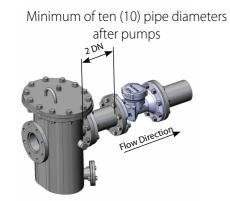
Minimum of two (2) pipe diameters after strainers
